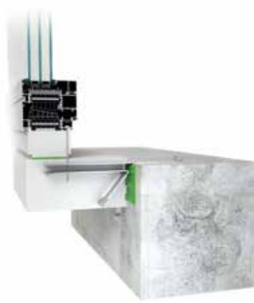
bottom connection, 200 mm beam with internal anchor
