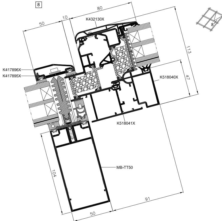
Transom and roof window - cross - section
