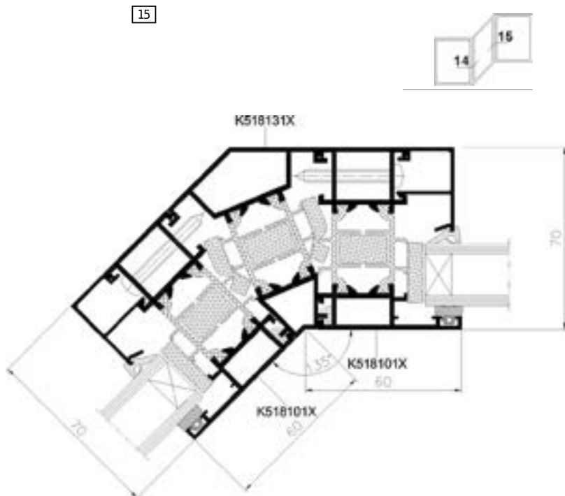
Angular connection - cross-section
